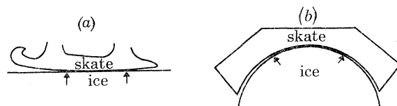
FIGURE 2. The contact between a curved skate and the ice surface in (a) real ice skating, (b) this experiment.
