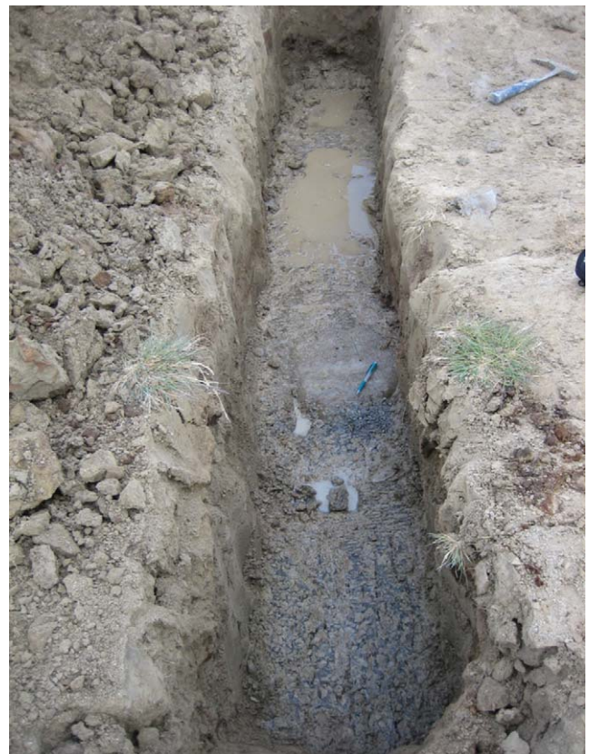
Fig. 4. Trench dug to establish ground truth on Devon Island. The trench shows a contact between permafrost (top of image) and wedge ice and then a contact between wedge ice and massive ice (dark, bottom of image) as marked by the tip of the pencil. The depth to the wedge ice is approximately 55 cm. The depth to the permafrost is 66 cm. A geologic hammer provides scale. Closer view of this contact may be seen in Fig. 6.
