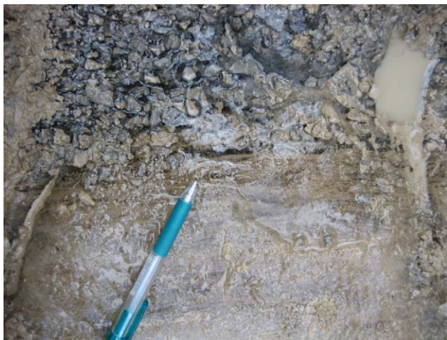
Fig. 5. Enlarged view of the contact between wedge ice (bottom) and massive ice (top) at Thomas Lee Inlet on Devon Island. Note the foliated texture of wedge ice. Both types of ice were mostly pure with fine soils included in the form of foliations (wedge ice) and blebs (massive ice). A mechanical pencil provides scale.
