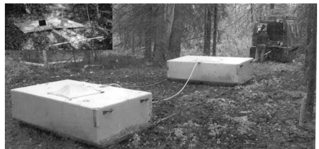
Figure 15. GSSI radar system including antennas and tracked vehicle. The prototype system is shown in the upper left.
